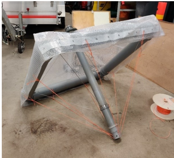
Figure 16 The structure of the gas-collecting hood.
