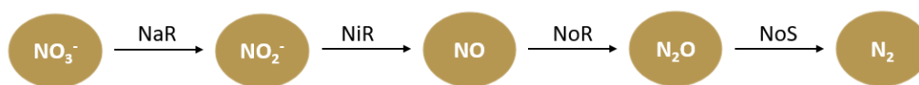
Figure 5 Heterotrophic denitrification as a pathway for N_2O emissions (adapted from Pijuan and Zhao, 2022).
